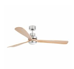
LANTAU XL is a modern ceiling fan with DC motor and a ground - breaking design, ideal for the ventilation of rooms over 17.6m2. Motor made of steel and wooden blades. Operated on remote control (included). It has 3 adjustable speeds with a 24 - 39 - 82W consumption and 70 - 95 - 135 revolutions per minute depending on speed. This fan comes with a reverse function, so you can also use it in winter, improving the efficiency of your heating system. This ceiling fan is suitable for inclining roof.
